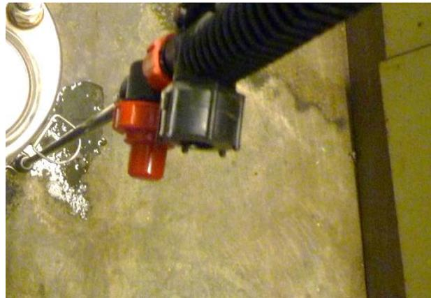
Leaked nozzles that needs to be replaced
